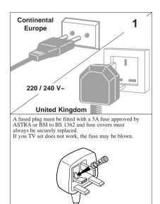
Note: The mains lead of the TV set is fitted with a moulded plug. Because it contains safety components we cannot recommend re-wiring.
